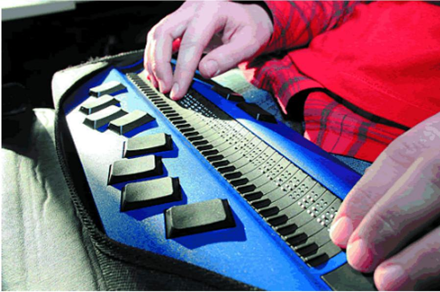
Figura 8.16: Exemplo de linha Braille (www.handytech.de (<http://www.handytech.de>))
