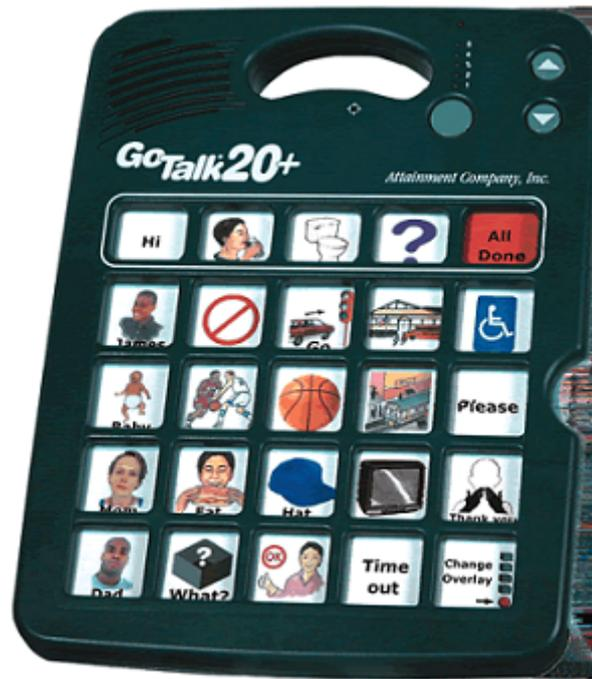
Figura 8.11: Digitalizadores de fala ([www.attainmentcompany.com](http://www.attainmentcompany.com))
