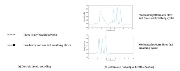
**Figure 5.** Examples of (a) discrete breath encoding, where soft and heavy breathing blows are recorded to encode combinations of zeros and ones, or Morse codes, representing the intended messages, and (b) continuous breath encoding, where the speed, amplitude, and phase of breathing are modulated to create patterns representing the intended message.
