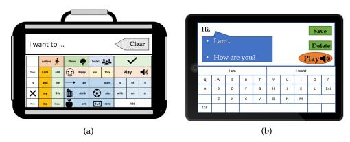
**Figure 4.** Examples of (a) a dedicated touch-based device and (b) a non-dedicated smart device running an AAC application (APP), usually with predictive language model and speech generation capabilities.
