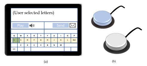
**Figure 3.** (a) A sample visual scanning interface activated via switch scanning. The yellow box moves vertically across the lines until a selection is made, followed by a gliding green box moving horizontally across the highlighted line until a letter is also selected. In (b), two scanning button switches are displayed.
