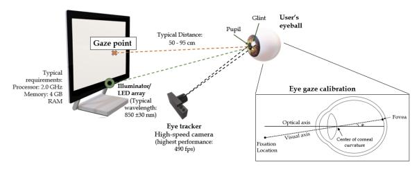
**Figure 2.** Components of a typical eye gaze system, adapted from [22,38]. The optical and the visual axes are used for the calibration process commonly required to set up the eye gaze system [22,39].
