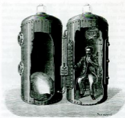
Figure 13.9 Figure from La pression barométrique 42 showing Paul Bert breathing oxygen while sitting in the chamber at progressively subatmospheric pressures. Note the sparrow in the cage above the subject – the bird falls in its cage when the pressure reaches 450 mmHg but Bert persists with the experiment down to 410 mmHg, maintaining consciousness by intermittently breathing oxygen. (Reproduced by permission of the Wellcome Library of the History of Medicine.)
